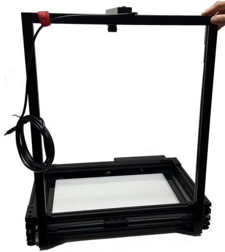
Figure 5: Camera mount in place
