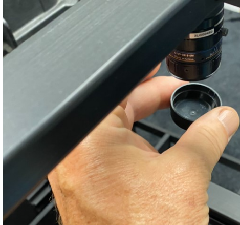
Figure 7: Removing black plastic lens cover
