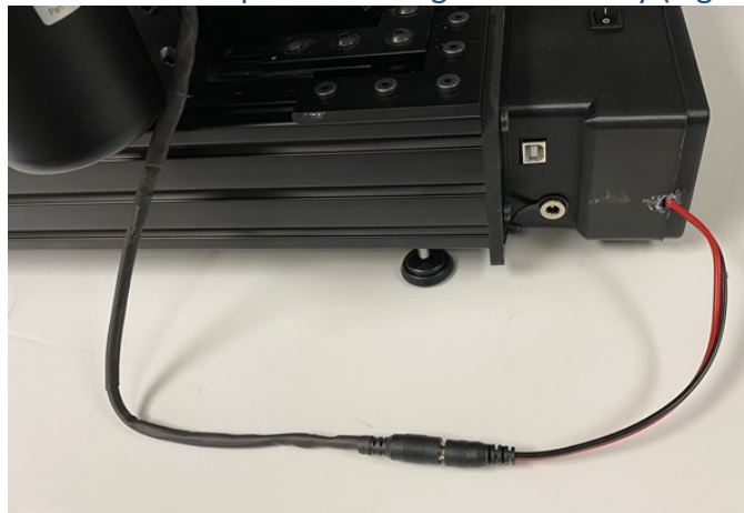
Figure 19: SIRTAKI motor connected to BASE controller
