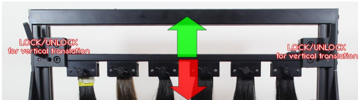
Figure 14: Swatches mount up or down
