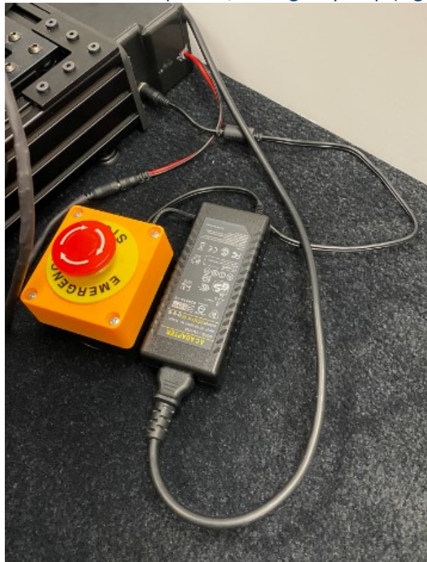
Figure 21: Base connected to DC power/ Emergency Stop
