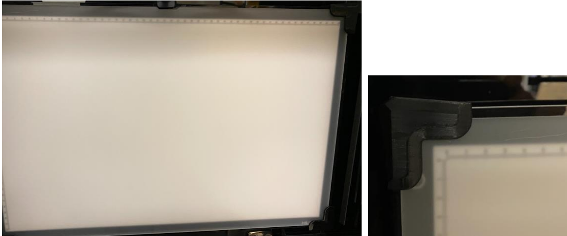
Figure 35: Diffusive matte panel on top of LED back panel
