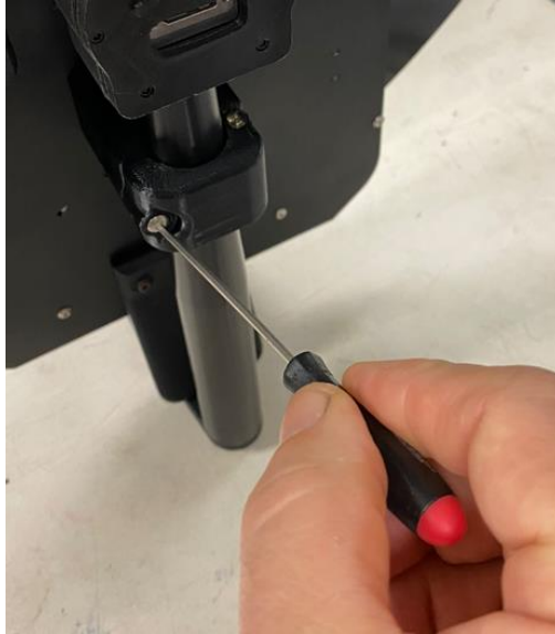
Figure 38: Securing RUMBA in place
