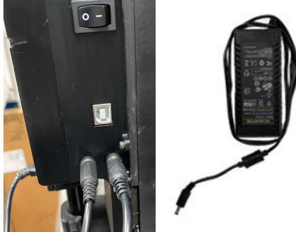
Figure 42: RUMBA connected to power supply
