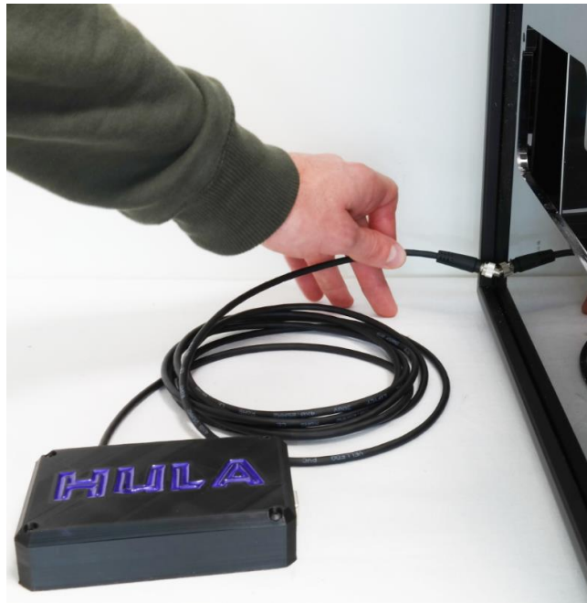
Figure 34: Cable on the side of the humidity box
