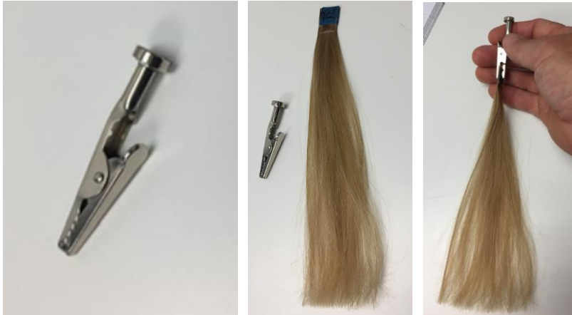
Figure 18: Mounting the hair swatch
