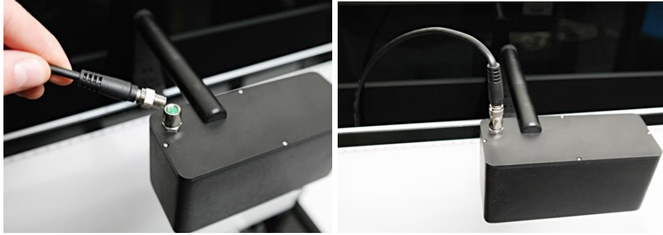
Figure 31: Connection between controller and hair swatch mount
