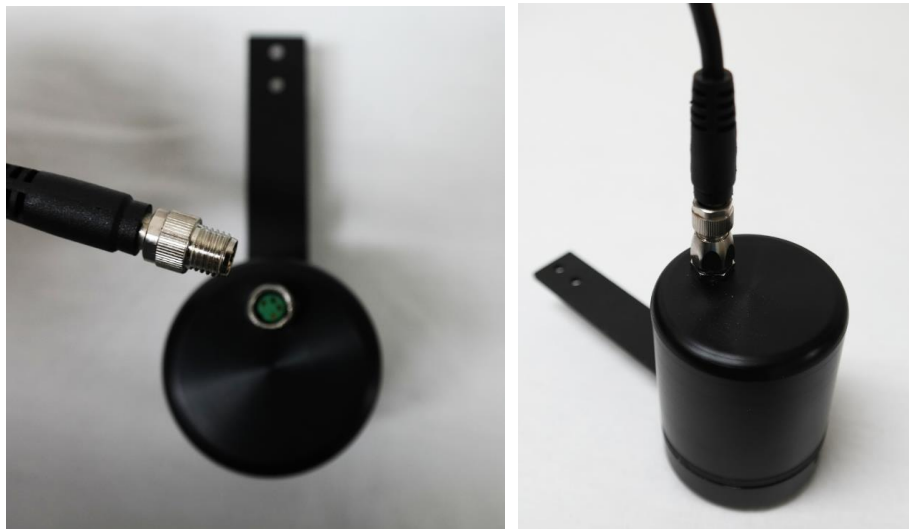
Figure 26: Connection between controller and hair swatch mount
